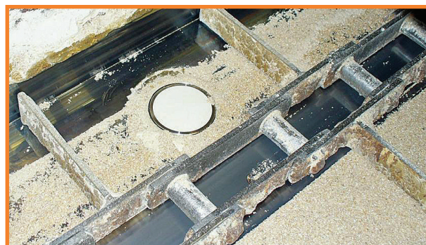
Measuring moisture of animal feed in conveyor
